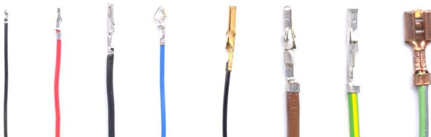
**FIG.8** Typical Molex Terminals Crimped on the Mini-Mac.
